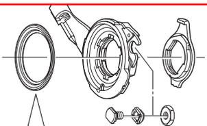
This cap is not required when combining CJ-NX10 with SG-7C21
